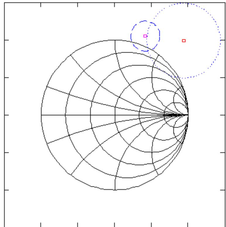
$$C_L = \frac{(S_{22} - \Delta S_{11}^*)^*}{|S_{22}|^2 - |\Delta|^2} = 1.361 \angle 47^\circ$$
